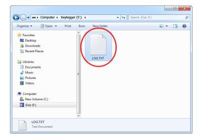
The removable disk will contain the file LOG.TXT with a text log of all captured data. Keystroke data is formatted in the same as it would appear on the screen, with special keys in brackets ([Ent], [Esc], [Del] etc.). This file can be viewed and searched with any text editor, such as *Notepad* or *MS Word*.
