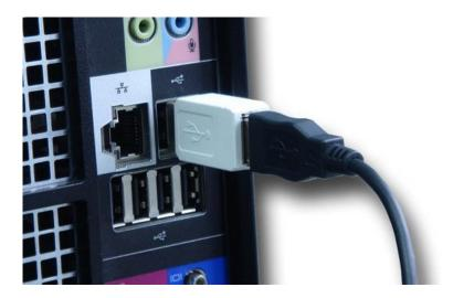
Connect the hardware USB keylogger between the USB keyboard and the USB port.
