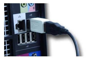
**To view recorded data**, plug the device in-between the keyboard and USB port, and press the 3-key combination **simultaneously** (by default K, B, S)
