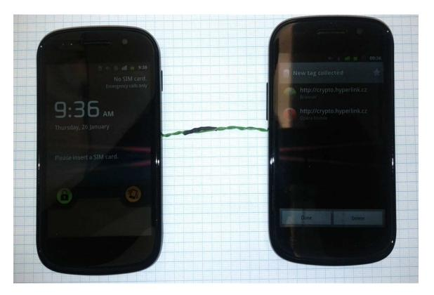
Two Google Nexus S (19023) with Android 2.3.6 working in reader-toreader mode (user tag transfer).
