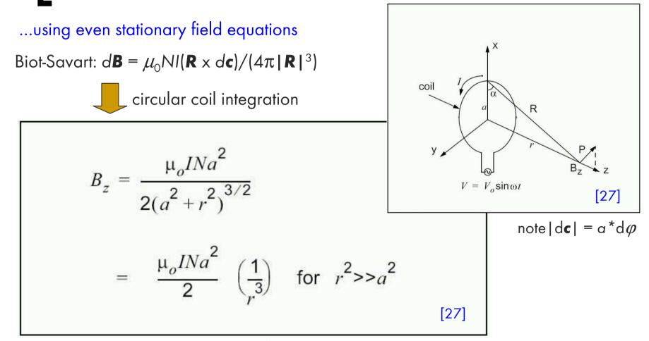
Optimum antenna diameter:  $a = r^* \sqrt{2}$ , where *r* is the communication distance.
