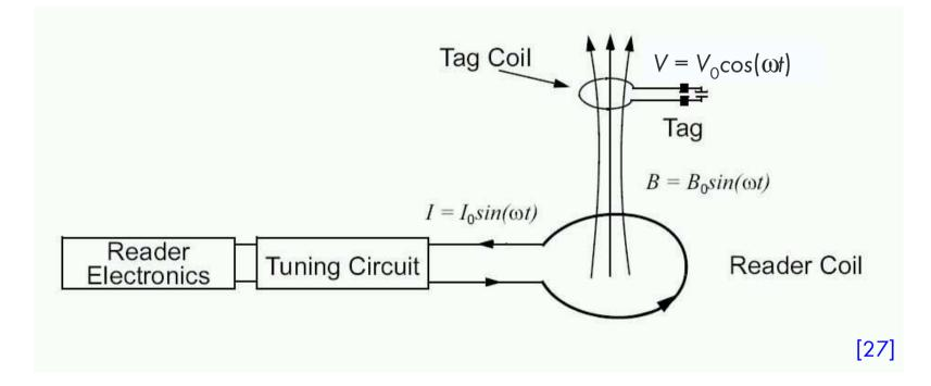
The tag itself is assumed to have no autonomous power source. It gets the energy for computation solely from the terminal's field.
