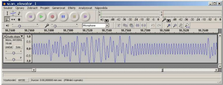
LF band transponder data intercepted while its holder was authenticating to the reader in an elevator. Distance: cca 0,5 m. Receiver: Sangean ATS 909W.
