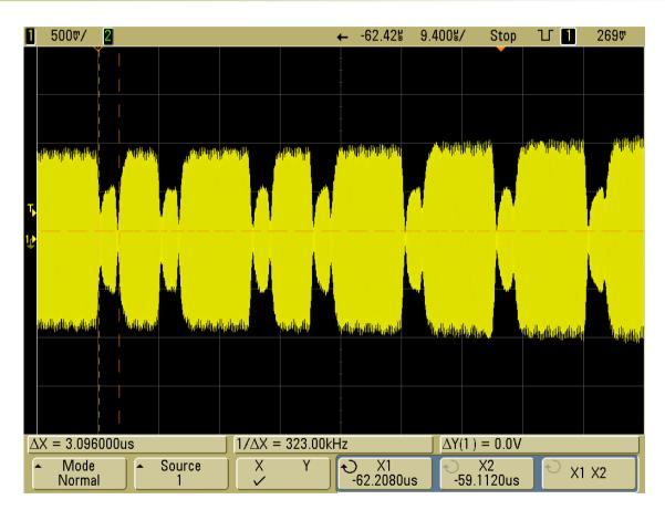
Receiver AOR AR8600MK2, HF output at i.f. 10,7 MHz. Distance cca 2 m, at least two readers in the field.
